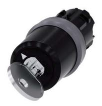
key-operated switch Siemens, 22 mm, round, plastic with metal front ring, lock number SSG10, with 2 keys, 2 switch positions O-I, latching, actuating angle 90°, 10:30h/13:30h, key removal O, Z=50-unit packaging
