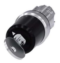
key-operated switch Siemens, 22 mm, round, metal, shiny, lock no. LSG1, with 2 keys, 2 switch positions O<I, momentary contact type, actuating angle 45°, 10:30h/12h, key removal O, with laser labeling, upper case and lower case, always upper case at the beginning of the word
