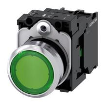
Illuminated pushbutton, 22 mm, round, Metal, shiny, green, pushbutton, flat, momentary contact type, with holder, 1NO, LED module with integrated LED 230 V AC, screw terminal, with laser labeling, symbol number according to, ISO 7000 or IEC 60417
