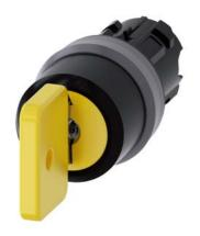
Key-operated switch O.M.R, 22 mm, round, plastic with metal front ring, lock number 73033, yellow, with 2 keys, 3 switch positions I-O-II, latching, actuating angle 2x45°, 10:30h/12h/13:30h, Key removal I+O+II, with laser labeling, upper case and lower case, always upper case at beginning of line
