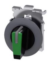
Selector switch, illuminable, 30 mm, round, Metal, matte, green, selector switch, short, front ring for flush installation, 3 switch positions I>O<II, momentary contact type, actuating angle 2x45°, 10:30h/12h/13:30h, with laser labeling, upper case and lower case, always upper case at beginning of line
