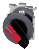
Selector switch, illuminable, 30 mm, round, Metal, matte, red, selector switch, long, front ring for flush installation, 2 switch positions O<I, momentary contact type, Actuating angle 45°, 10:30h/12h, with laser labeling, inscription or symbol Customer-specific selection with SIRIUS ACT configurator (CIN)
