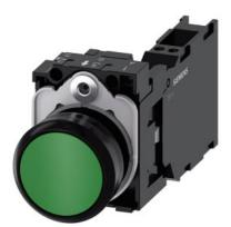
Pushbutton, 22 mm, round, plastic, green, pushbutton, flat, momentary contact type, with holder 1 NO+1 NC, spring-type terminal, with laser labeling, lower case
