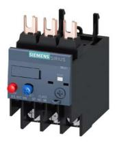
Overload relay 5.5...8.0 A Thermal For motor protection Size S0, Class 10 Contactor mounting Main circuit: Ring cable lug Auxiliary circuit: ring cable lug Manual-Automatic-Reset
