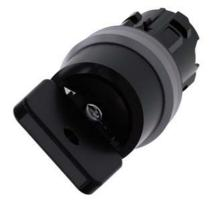
Key-operated switch O.M.R, 22 mm, round, plastic with metal front ring, lock number 73034, black, with 2 keys, 2 switch positions O<I, momentary contact type, Actuating angle 45°, 10:30h/12h, key removal O, with laser labeling, upper case and lower case, always upper case at beginning of line
