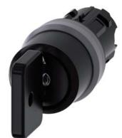
Key-operated switch O.M.R, 22 mm, round, plastic with metal front ring, lock number 73034, black, with 2 keys, 3 switch positions I-O<II, left latching, right momentary contact type, actuating angle 2x45°, 10:30h/12h/13:30h, key removal I, with laser labeling, lower case
