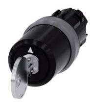
Key-operated switch BKS, 22 mm, round, plastic with metal front ring, lock number S1, with 2 keys, 3 switch positions I-O-II, latching, actuating angle 2x45°, 10:30h/12h/13:30h, key removal I, with laser labeling, inscription or symbol Customer-specific selection with SIRIUS ACT configurator (CIN)
