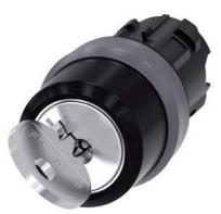
RONIS key-operated switch, 22 mm, round, plastic with metal front ring, lock number 455, with 2 keys, 2 switch positions O-I, latching, actuating angle 90°, 10:30h/13:30h, key removal O, with laser labeling, inscription or symbol Customer-specific selection with SIRIUS ACT configurator (CIN)
