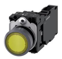
Illuminated pushbutton, 22 mm, round, plastic with metal front ring, yellow, pushbutton, flat, momentary contact type, with holder, 1 NO+1 NC, LED module with integrated LED 24 V AC/DC, screw terminal, with laser labeling, upper case and lower case, always upper case at beginning of line
