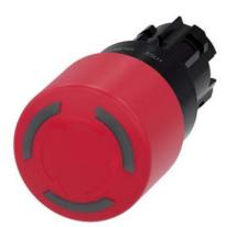
EMERGENCY STOP mushroom pushbutton, illuminable, 22 mm, round, plastic, red, 30 mm, positive latching, acc. to EN ISO 13850, rotate-to-unlatch, with laser labeling, lower case
