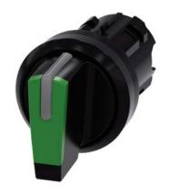
Selector switch, illuminable, 22 mm, round, plastic, green, selector switch, short, 3 switch positions I-O-II, latching, actuating angle 2x45°, 10:30h/12h/13:30h, with laser labeling, upper case and lower case, always upper case at the beginning of the word
