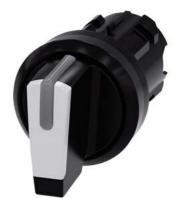
Selector switch, illuminable, 22 mm, round, plastic, white, selector switch, short, 3 switch positions I>O<II, momentary contact on the left, latching on the right, actuating angle 2x45°, 10:30h/12h/13:30h, with laser labeling, upper case and lower case, always upper case at the beginning of the word
