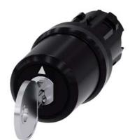
key-operated switch Siemens, 22 mm, round, plastic, lock number SSG10, with 2 keys, 3 switch positions I-O-II, latching, actuating angle 2x45°, 10:30h/12h/13:30h, key removal O, with laser labeling, upper case and lower case, always upper case at beginning of line
