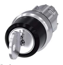
RONIS key-operated switch, 22 mm, round, metal, shiny, lock number SB30, with 2 keys, 3 switch positions I>O<II, momentary contact type, actuating angle 2x45°, 10:30h/12h/13:30h, key removal O, possible special locks: SB31, 421, 455, with laser labeling, upper case and lower case, always upper case at beginning of line
