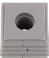
Seal, Mounting type: Plug in, Length x width: 20.3 mm, Max. cable diameter: 9 mm, IP 66, Colour: Grey
