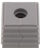
Seal, Mounting type: Plug in, Length x width: 20.3 mm, Max. cable diameter: 8 mm, IP 66, Colour: Grey
