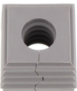
Seal, Mounting type: Plug in, Length x width: 20.3 mm, Max. cable diameter: 10 mm, IP 66, Colour: Grey
