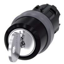
RONIS key-operated switch, 22 mm, round, plastic with metal front ring, special lock, with 2 keys, 3 switch positions I-O-II, latching, actuating angle 2x45°, 10:30h/12h/13:30h, key removal O+I, possible special locks: SB31, 421, 455
