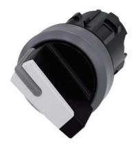
Selector switch, illuminable, 22 mm, round, plastic with metal front ring, white, selector switch, short, 2 switch positions O-I, latching, actuating angle 90°, 10:30h/13:30h, Z=50-unit packaging
