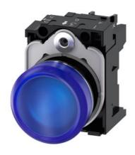
Indicator light, 22 mm, round, metal, shiny, blue, lens, smooth, with holder, LED module with integrated LED 110 V AC, screw terminal, with laser labeling, upper case and lower case, always upper case at beginning of line
