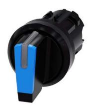
Selector switch, illuminable, 22 mm, round, plastic, blue, selector switch, short, 3 switch positions I-O-II, latching, actuating angle 2x45°, 10:30h/12h/13:30h, with laser labeling, upper case
