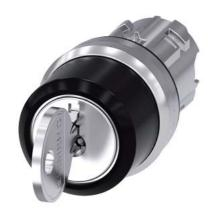
RONIS key-operated switch, 22 mm, round, metal, shiny, lock number 455, with 2 keys, 3 switch positions I-O-II, latching, actuating angle 2x45°, 10:30h/12h/13:30h, Key removal I+O+II, with laser labeling, inscription or symbol Customer-specific selection with SIRIUS ACT configurator (CIN)
