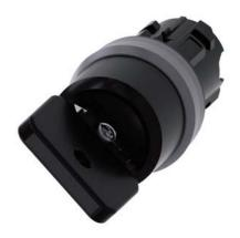
Key-operated switch O.M.R, 22 mm, round, plastic with metal front ring, lock number 73034, black, with 2 keys, 2 switch positions O-I, latching, actuating angle  $90^\circ,\,10:\!30h/13:\!30h,$  key removal O, with laser labeling, upper case and lower case, always upper case at beginning of line
