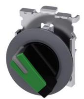
Selector switch, illuminable, 30 mm, round, Metal, matte, green, selector switch, short, front ring for flush installation, 2 switch positions O-I, latching, actuating angle  $90^{\circ}$ , 10:30h/13:30h, with laser labeling, lower case
