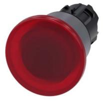
Illuminated mushroom pushbutton, 22 mm, round, plastic with metal front ring, red, 40mm, latching, pull-to-unlatch mechanism, with laser labeling, upper case and lower case, always upper case at beginning of line
