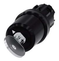
Key-operated switch BKS, 22 mm, round, plastic, lock number S1, with 2 keys, 2 switch positions O<I, momentary contact type, Actuating angle 45°, 10:30h/12h, Key removal O Z=50-unit packaging
