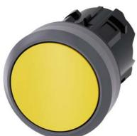
Pushbutton, 22 mm, round, plastic with metal front ring, yellow, pushbutton, flat, latching, Push-to-release mechanism, Z=100-unit packaging
