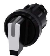
Selector switch, illuminable, 22 mm, round, plastic, white, selector switch, short, 3 switch positions I>O<II, momentary contact on the left, latching on the right, actuating angle  $2x45^{\circ}$ , 10:30h/12h/13:30h, with laser labeling, upper case and lower case, always upper case at beginning of line
