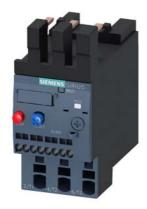
Overload relay 14...20 A Thermal For motor protection Size S0, Class 10 Contactor mounting Main circuit: Spring-type terminal Auxiliary circuit: spring-type terminal Manual-Automatic-Reset
