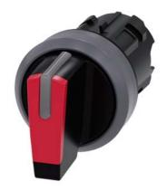
Selector switch, illuminable, 22 mm, round, plastic with metal front ring, red, selector switch, short, 3 switch positions I>O<II, momentary contact on the left, latching on the right, actuating angle 2x45°, 10:30h/12h/13:30h, with laser labeling, upper case and lower case, always upper case at beginning of line
