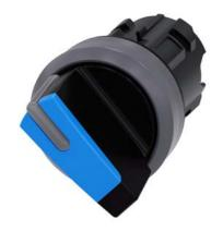
Selector switch, illuminable, 22 mm, round, plastic with metal front ring, blue, selector switch, short, 2 switch positions O<I, momentary contact type, Actuating angle 45°, 10:30h/12h, with laser labeling, inscription or symbol Customer-specific selection with SIRIUS ACT configurator (CIN)
