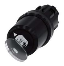
Key-operated switch BKS, 22 mm, round, plastic, Lock No. E7 (VW), without key, 2 switch positions O-I, latching, actuating angle 90°, 10:30h/13:30h, key removal O+I, with laser labeling, upper case
