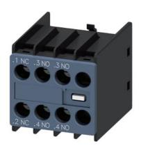
Auxiliary switch on the front, 2 NO + 1 NC Current path 1 NC, 1 NO, 1 NO for 3RH and 3RT screw terminal .1/.2, .3/.4, .3/.4
