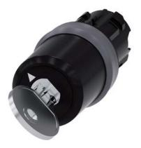
Key-operated switch BKS, 22 mm, round, plastic with metal front ring, Lock No. E9 (VW), without key, 2 switch positions O-I, latching, actuating angle  $90^{\circ}$ , 10:30h/13:30h, key removal O, Z=50-unit packaging
