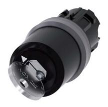
Key-operated switch IKON, 22 mm, round, plastic with metal front ring, lock number 360012K1, with 2 keys, 2 switch positions O-I, latching, actuating angle 90°, 10:30h/13:30h, key removal O+I, Z=50-unit packaging
