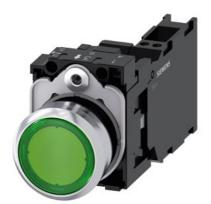
Illuminated pushbutton, 22 mm, round, metal, shiny, green, pushbutton, flat, momentary contact type, with holder, 1 NO+1 NC, LED module with integrated LED 24 V AC/DC, spring-type terminal, with laser labeling, upper case
