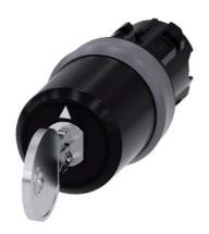
Key-operated switch BKS, 22 mm, round, plastic with metal front ring, lock number S1, with 2 keys, 3 switch positions I-O-II, latching, actuating angle 2x45°, 10:30h/12h/13:30h, Key removal II, Z=50-unit packaging
