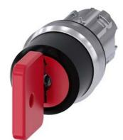
Key-operated switch O.M.R, 22 mm, round, metal, shiny, lock number 73037, red, with 2 keys, 3 switch positions I-O-II, latching, actuating angle 2x45°, 10:30h/12h/13:30h, Key removal I+O+II, with laser labeling, lower case
