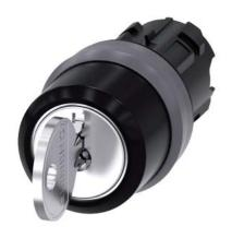
RONIS key-operated switch, 22 mm, round, plastic with metal front ring, lock number SB30, with 2 keys, 3 switch positions I-O-II, latching, actuating angle 2x45°, 10:30h/12h/13:30h, key removal O+I, possible special locks: SB31, 421, 455, with laser labeling, lower case
