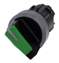
Selector switch, illuminable, 22 mm, round, plastic with metal front ring, green, selector switch, short, 2 switch positions O<I, momentary contact type, Actuating angle 45°, 10:30h/12h, with laser labeling, upper case and lower case, always upper case at the beginning of the word
