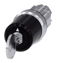
Key-operated switch BKS, 22 mm, round, metal, shiny, lock number S1, with 2 keys, 3 switch positions I>O<II, momentary contact on the left, latching on the right, actuating angle  $2x45^{\circ}$ , 10:30h/12h/13:30h, key removal O, with laser labeling, upper case
