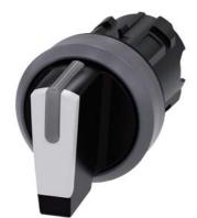
Selector switch, illuminable, 22 mm, round, plastic with metal front ring, white, selector switch, short, 3 switch positions I>O<II, momentary contact type, actuating angle  $2x45^{\circ}$ , 10:30h/12h/13:30h, with laser labeling, upper case
