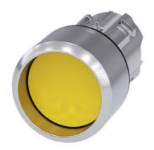
Pushbutton, 22 mm, round, metal, shiny, yellow, Front ring, high, momentary contact type, with laser labeling, lower case
