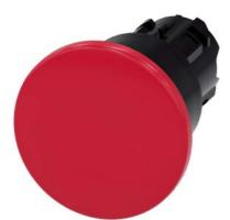
Mushroom pushbutton, 22 mm, round, plastic, red, 40mm, latching, pull-tounlatch mechanism, with laser labeling, symbol number according to, ISO 7000 or IEC 60417
