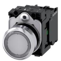
Illuminated pushbutton, 22 mm, round, Metal, shiny, transparent, pushbutton, flat, momentary contact type, with holder, 1NO, LED module with integrated LED 230 V AC, screw terminal, with laser labeling, upper case and lower case, always upper case at beginning of line
