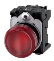
Indicator lights, 22 mm, round, Metal, shiny, red, lens, smooth, with holder, LED module with integrated LED 230 V AC, screw terminal, with laser labeling, lower case
