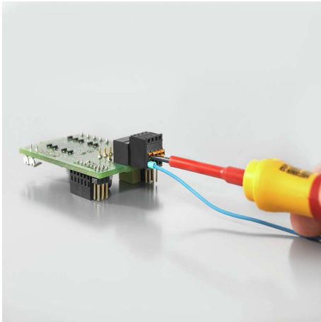
Operating safety Through PUSH IN connection system
