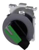
Selector switch, illuminable, 30 mm, round, Metal, matte, green, selector switch, long, front ring for flush installation, 2 switch positions O-I, latching, actuating angle 90°, 10:30h/13:30h, with laser labeling, upper case and lower case, always upper case at beginning of line
